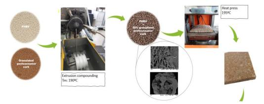
The cork (alveolar part) was successfully incorporated into the PHBV material, showing no signs of adhesion problems. The pellets exhibited a uniform appearance, indicating successful incorporation. Analysis of SEM images further confirmed the robust adhesion between PHBV and cork, with minimal occurrence of cavities or holes that could impede the processing phase.
